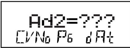
On your DT300 & DT400 throttles, the display will show Ad2 for two digit addresses and Ad4 for four digit addresses. All other CVs are displayed as numbers on Digitrax throttles. Be sure that CV29 is programmed to a value that has either "0" or "1" as the first digit to enable 2 digit addressing. See CV29 below for more information.
