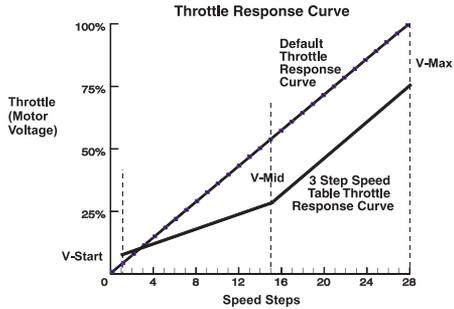
NOTE: Digitrax FX and later model decoders use V-start in 128 speed step mode and run loadable speed tables in 128 speed step mode. Other standard and most non-FX decoders disregard V-start in 128 speed step mode and run loadable speed tables in 14 or 28 speed step mode.
