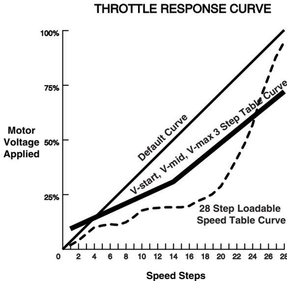
When you are using a throttle to control a locomotive, you will notice that as you increase and decrease the speed, the loco responds to the change in throttle settings according to the relationship between motor voltage applied and the throttle setting. This is called the throttle response curve. Decoders are shipped from the factory with a linear throttle response curve. This means
