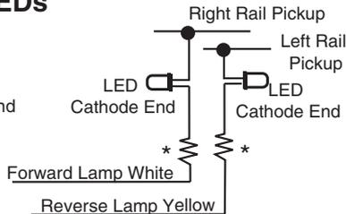
\* Note: LEDs are sensitive to polarity when hooked up. Typical resistor 680 ohm 1/4 watt.
