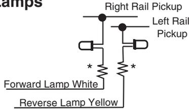
\* Note: Current setting resistor to suit the lamp used. Typically 560 ohm 1/4 watt for grain of rice and 250 ohm 1/4 watt for grain of wheat. Lower resistance values will increase the lamp brightness, minimum value is 100 ohms.
