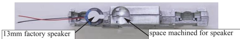
**Figure 3:** SDN144K1E Decoder installation in Kato SD40-2 - reassembly.
