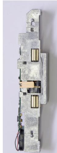
Figure 6: SD70ACE- showing a 10x18mm speaker in upper rear.
