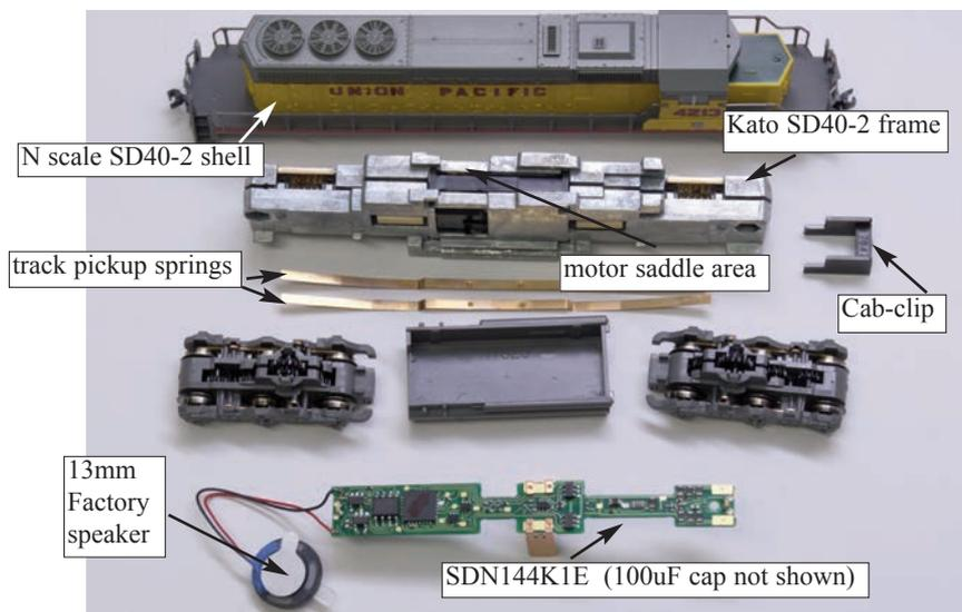
1. Carefully remove the Kato SD40-2 shell parts. Remove the factory analog light PCB, trucks, drive shafts, motor and all parts and carefully save these in the correct order for re-installation. This should leave a bare frame ready to be modified to accommodate the speaker.
