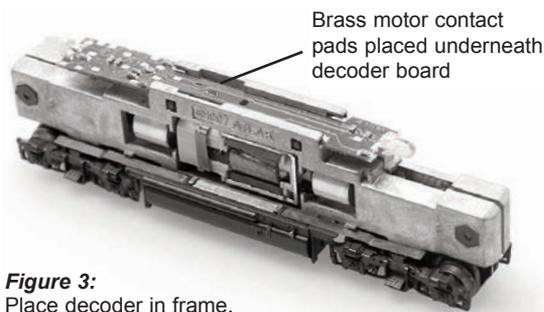
**Figure 3:** Place decoder in frame.
