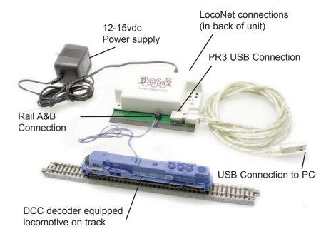
The connection diagram on following page will help you install the hardware correctly. Assemble the PR3 hardware as shown and connect to an appropriate power supply (Digitrax **PS14** or equivalent). Note the LocoNet output for MS100 operation, and the separate track output for SoundFX programming operations.
