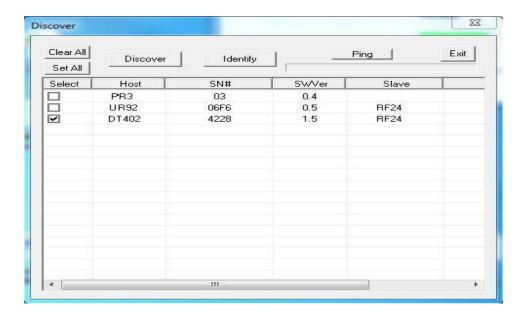
Again, use the scroll bar at the bottom of the Discover box to scroll all the way to the right.
