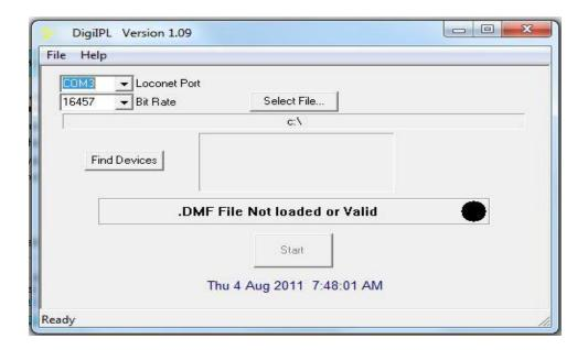
Verify that the proper LocoNet Port is selected. This is the Com Port that the computer has assigned to the PR3. The Bit Rate should be set for 16457.
