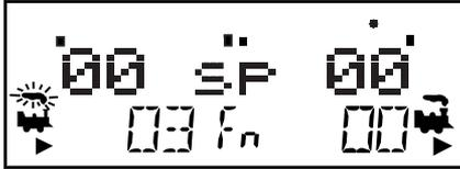
*The illustration above shows the LCD after address “00” is selected on the R Throttle Knob and address “03” is selected on the L Throttle Knob. We see the Power On Indicator in the top line, the speed bar graphs at 0 speed and the text area also at 0 speed for both throttles.*
