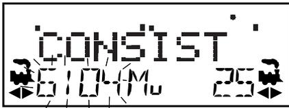
the MU mode indicator on the LCD display is lit. The loco address in the L side of the display will blink to show that it is the address that will be consisted to the address on the R Throttle.
