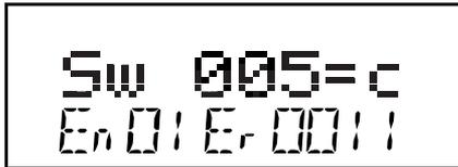
This display shows Entry 01, Route 11 with turnout address 005 set for closed. In this case address 005 is the TOP address for this route because it is Entry 01 for the Route.
