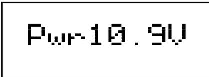
When you insert a battery or unplug from LocoNet, the value displayed will be the battery power. When this number is less than 6.2 V you may want to consider changing the battery. The DT400/R will still continue to
