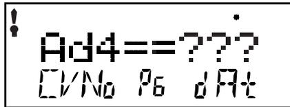
You can toggle between 2 & 4 digit address programming by pressing down on the R Throttle Knob.
