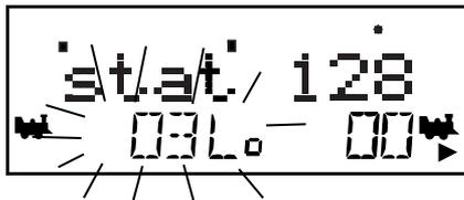
4. Press the LOCO Key
