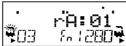
5. The DT400/R will use the **LocoNet ID** of the LocoNet it was plugged in to and will begin to operate as an IR throttle when you unplug it from LocoNet. When you unplug from LocoNet, the tetherless indicator will come on and the tetherless message will display for a few seconds indicating whether the throttle is running as Ir (infrared) or rA (radio). It will also display the LocoNet ID that the throttle is logged on to.
