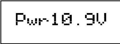
This screen indicates the power available to the throttle. When you are plugged in to LocoNet, this value will be between 9 & 15 volts. when
