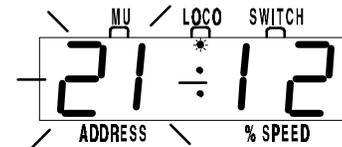
This display shows locomotive address 21 selected but not set, since the address 2 digits are flashing. Notice the status "12" indicates this address is common, 14 speed step mode.
