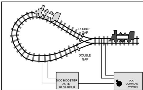
Note that when the polarity change occurs, DCC equipped locos will continue at the speed & in the direction commanded but any analog engines running will reverse direction because they see the polarity change & respond to it.
