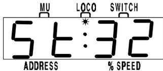
In this example the 3 means the Loco is in-use and the DT100 will not allow you to select this normally. The 2 means that this loco is being handled by the system as a 14 step decoder on the track.
