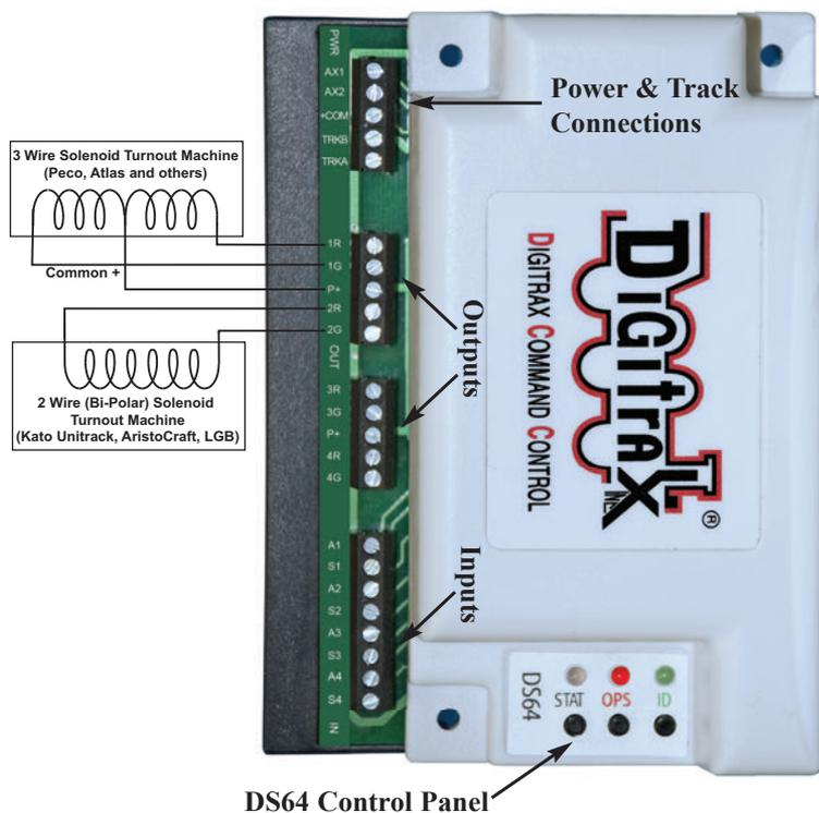
Note: Multiple turnout machines can be operated on a single DS64 output. For example, you can run 2 Peco or Atlas Snap Switches on a single DS64 output. Up to 4 Kato Unitrack switches (such as the Unitrack double crossover) can be operated a on a single DS64 output.
