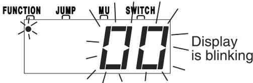
5. Use the numeric keypad to enter "03", the address used to control the locomotive with the decoder. Your display will show:
