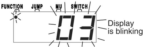
6. Press the **LOCO** key again to confirm your selection and set address 03 on the throttle. The display will stop blinking and you will have control of the DCC equipped locomotive with address 03.
