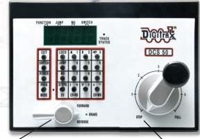
**Direction/Brake** lever in "BRAKE" position
