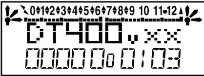
This screen shows the DT400's software version number. It is displayed for a few seconds each time you power on the DT400.
