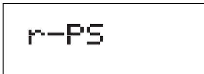
The throttle may flash the normal Fn Mode screen about every 60 seconds. This happens when the throttle “pings” the system to let the command station know that it is still part of the system. This keeps the system from releasing that locomotive back to the system and making it available to be selected by another throttle.
