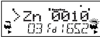
This example shows a DT400 in FIND mode for address 1652 selected on the R Throttle. The system sees address 1652 in Zone 0010. When address 1652 moves to another Zone, the display will automatically update to show the new Zone location.
