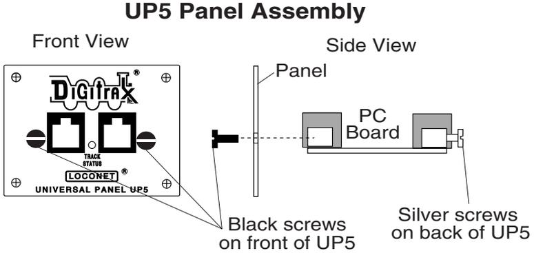
Universal panels are shipped without front fascia panels attached. Simply use the screws provided to attach this panel to the PC board as shown above. The diagram below shows how to hook up your UP panel on your layout. Instructions are also included below for hooking up the track status indicator. This is an optional feature and the UPs will work just fine even if you do not hook up the track status indicator to the local track section.
