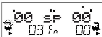
The illustration above shows the LCD after address “00” is selected on the R Throttle and address “03” is selected on the L Throttle, We see the Power On Indicator in the top line, the speed bar graphs at 0 speed and the text area also at 0 speed for both throttles.
