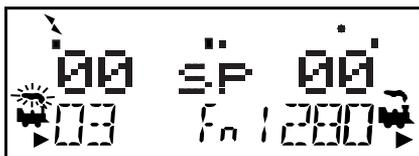
If an untethered DT400/R, operating as a tetherless throttle, detects no user throttle activity for about 3 minutes it will enter power save mode. The display will show:
