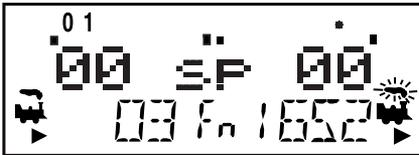
This screen displays current addresses selected on the L & R throttles along with their current speed and direction. The functions that are turned ON for the active throttle (the one with the blinking smoke icon) are displayed across the top of the display.
