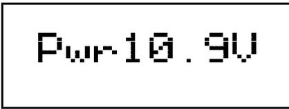
When you insert a battery or unplug from LocoNet, the value displayed will be the battery power. When this number is less than 6.2 V you may want to consider changing the battery. The DT400/R will still continue to
