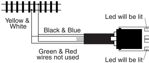
You can also use a bi-color LED indicator lamp, with a 500 to 1k ohm resistor in series, connected to the two rails of the powered track.
