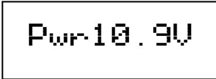
This screen indicates the power available to the throttle. When you are plugged in to LocoNet, this value will be between 9 & 15 volts. when you insert a battery or unplug from LocoNet,
