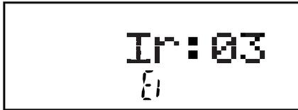
This display shows a DT400 that has found an Infrared receiver on LocoNet with a current LocoNet ID of 03. The DT400 is ready to Edit the LocoNet ID. Other characters may be displayed on the screen at this time depending on the current throttle state.
