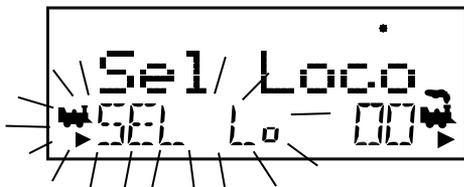
*The illustration above shows the LCD display just after you press the LOCO Key to select an address on the L Throttle when nothing has been selected on that throttle before and where address "00" is selected to run on the R Throttle.*
