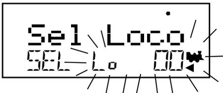
*This illustration shows what will be on your LCD when you press the LOCO Key to select an address on the R Throttle if address “00” was the last address selected on the R Throttle and where no address has been previously selected for the L Throttle.*
