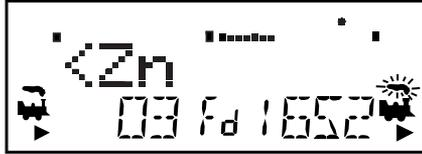
This example shows a DT400 in FIND mode for address 03 selected on the L Throttle. The system is not able to find address 03 so there is no display after the <Zn. Either the loco or rolling stock with address 03 is not present on the layout or it does not have a transponder or it is located in a zone that does not have a transponder receiver.
