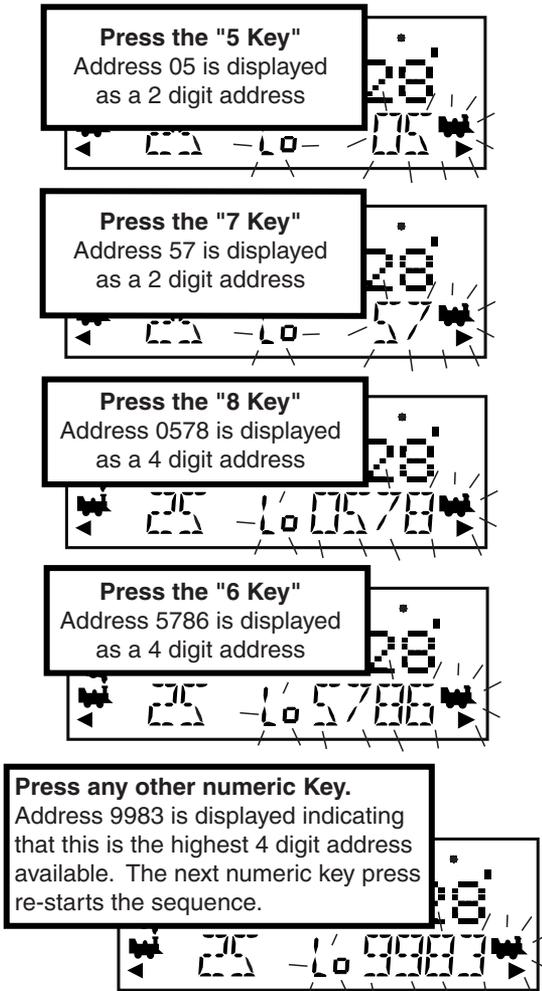
4. To select a 2 digit address, use the keypad to enter the address of the loco you want to run OR turn the L throttle knob counterclockwise until you see 00 appear in the display, then use the R throttle knob to dial up a 2 digit address between 00 & 127.
