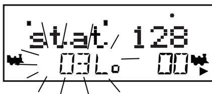
*The illustration above shows the LCD display as you browse through decoder addresses. The display shows the decoder address and its decoder status. See Section 17 for more information about decoder status.*
