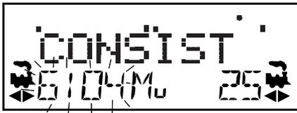
the MU mode indicator on the LCD display is lit. The loco address in the L side of the display will blink to show that it is the address that will be consisted to the address on the R Throttle.
