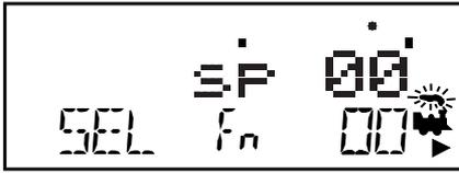
*This illustration shows the LCD after pressing the LOCO Key to complete the selection process. Loco address 00 is selected on the R Throttle and is not moving.*
