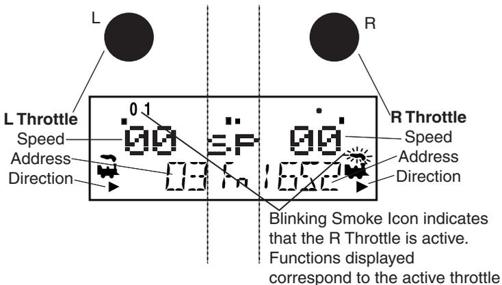
1. The DT400 handheld has two throttles called the Left throttle (L) and the Right throttle (R).
