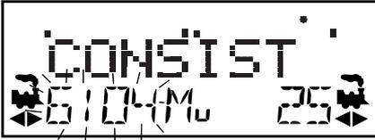
the MU mode indicator on the display is lit. The loco address in the **L** side of the display will blink to show that it is the address that will be consisted to the address on the **R** Throttle.
