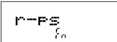
The throttle may flash the Fn mode indicator about every 60 seconds. This
