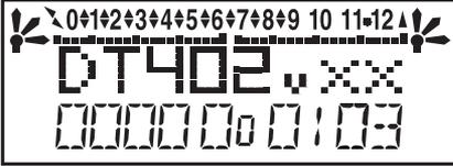
This screen shows the throttle type (v): DT402, DT402R or DT402D and software version number (xx). It is displayed for a few seconds each time you power on the DT402.
