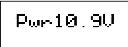
This screen indicates the power available to the throttle. When you are plugged in to LocoNet, this value should be between 9 and 15 volts for proper operation. When you insert a battery or unplug from LocoNet, the value displayed shows the battery power available. When this number is less than 6.2 volts it's time to replace the battery. *See Section 3.0 for more information about installing/replacing the batteries in your DT402.*
