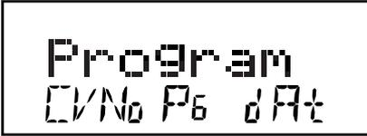
“CVNo” on the left side indicates that configuration variable numbers will show on the left and “dAt” on the right side indicates that CV values or data will show on the right side of the display.
