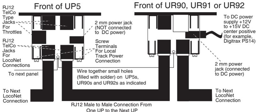
Note: You can run up to 10 UP or UR panels with a single DC power supply by simply connecting the small holes on each panel as indicated in this diagram.
