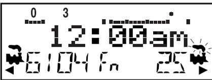
Any DT series throttle (including your DT402) that is plugged in to your LocoNet system will update its fast clock time and rate to be synchronized to the rest of the system a couple of seconds after it is connected to LocoNet.
