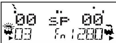
If an untethered DT402R operating as a tetherless throttle detects no user throttle activity for about 3 minutes, it will enter power save mode. You will see:
