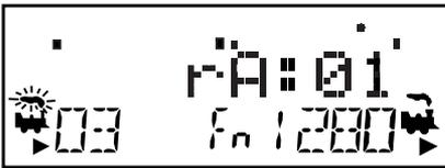
3. Unplug the DT402R from the LocoNet. The tetherless indicator on the display will come on and the tetherless message will display for a few seconds indicating whether the throttle is running in rA (radio) mode. It will also display the LocoNet ID (00-07) that the throttle is logged on to.
