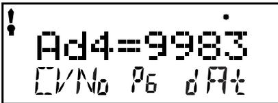
Alternatively, you can use the DT402's Throttle Knobs to dial in the 4 digit address you want to program. Use the **L** Throttle to dial up 1000s and 100s and the **R** Throttle to dial up 10s and 1s. Press the **ENTER** key to program the decoder
