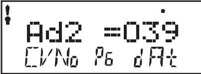
Note, when programming a 2-digit address, the decoder automatically enables 2-digit addressing.
