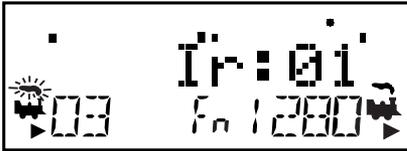
3. Unplug the DT402 from the LocoNet. The tetherless indicator on the display will come on and the tetherless message will display for a few seconds indicating whether the throttle is running in Ir (infrared) mode. It will also display the LocoNet ID (00-07) that the throttle is logged on to.
