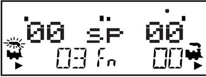
7. Turn the **L** Throttle knob clockwise slowly to increase the speed of the decoder equipped locomotive. As the value in the left display increases, the decoder equipped locomotive on the track will begin to move.
