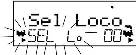
5. Use the numeric keypad to enter 03 or use the **R** Throttle knob to select Address “03” in the left side of the display. (The **R** Throttle knob changes 1s and 10s, the **L** Throttle knob changes 100s and 1000s.)
