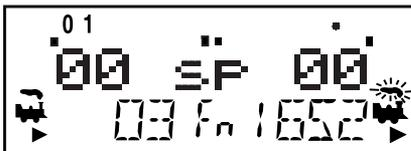
This screen displays current addresses selected on the L and R throttles along with their current speed and direction. The functions that are turned ON for the active throttle (the one with the blinking smoke icon) are displayed across the top of the display.
