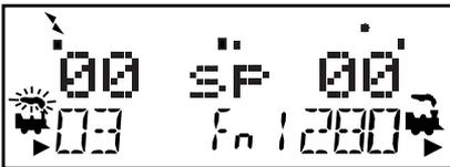
If an untethered DT402 operating as a tetherless throttle detects no user throttle activity for about 3 minutes, it will enter power save mode. The display will show:
