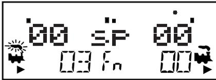
7. Turn the **L** Throttle knob clockwise slowly to increase the speed of the decoder equipped locomotive. As the value in the left display increases, the locomotive on the track will begin to move.
