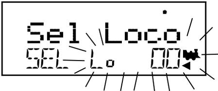
5. Press the **LOCO** key again to select address 00 on the throttle. You can also press the **R** Throttle knob once to select the loco address and return to Fn mode for normal operation.
