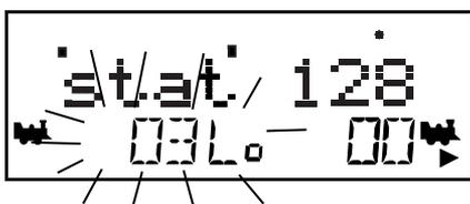
6. Press the **LOCO** key again to select address 03 on the throttle. You can also press the **L** Throttle knob once to select the loco address and return to Fn mode for normal operation.
