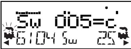
6. Key in the number of the OpSw. In the example above, we have keyed in 5 for the switch. As you browse through the OpSw's, the right side of the text area will show the current setting for each OpSw, either "c" or "t".
