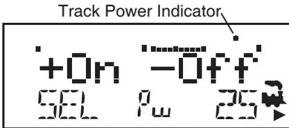
2. Press the **N / -** key to toggle the track power off. The TRACK POWER Indicator on your DT402 and on your Command Station will go off.
