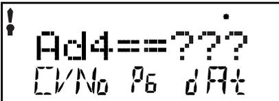
You can toggle between 2- and 4-digit address programming by pressing down on the **R** Throttle knob.
