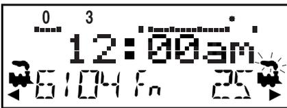
Any DT series throttle (including your DT402) that is plugged in to your LocoNet system will update its fast clock time and rate to be synchronized to the rest of the system a couple of seconds after it is connected to LocoNet.
