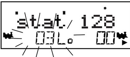
6. Press the **LOCO** key again to select address 03 on the throttle. You can also press the **L** Throttle knob once to select the loco address and return to Fn mode for normal operation.
