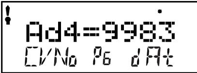
3. Select the programming mode you wish to use by pressing the **PROG** key until the method you want appears in the Mode Indicator. Digitrax recommends using the Pd, or Direct mode for programming Digitrax decoders when using service mode on the programming track.
