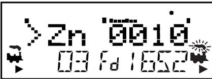
This example shows a DT402 in FIND mode for address 1652 selected on the **R** Throttle. The system sees address 1652 in Zone 0010 moving at about 50% of full throttle. When address 1652 moves to another Zone, the display will automatically update to show the new Zone location.
