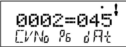
Remember that you can press the **R** Throttle knob to toggle the CV value display between decimal and hex as shown below.
