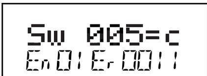
This display shows Entry 01, Route 11 with turnout address 005 set for **c** (closed). In this case address 005 is the TOP address for this route because it is Entry 01 for the Route.
