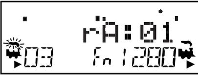
3. Unplug the DT402R from the LocoNet. The tetherless indicator on the display will come on and the tetherless message will display for a few seconds indicating whether the throttle is running in rA (radio) mode. It will also display the LocoNet ID (00-07) that the throttle is logged on to.
