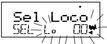
5. Press the **LOCO** key again to select address 00 on the throttle. You can also press the **R** Throttle knob once to select the loco address and return to Fn mode for normal operation.
