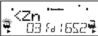
This example shows a DT402 in FIND mode for address 03 selected on the **L** Throttle. The system is not able to find address 03 so there is no display after the <Zn. Either the loco or rolling stock with address 03 is not present on the layout or it does not have a transponder or it is located in a zone that does not have a transponder receiver.
