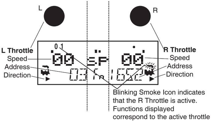
1. The DT402 handheld has two knobs called the **L Throttle** (Left) and the **R Throttle** (Right). The throttles are used for speed control, direction changes, and input of information for operation of your railroad.
