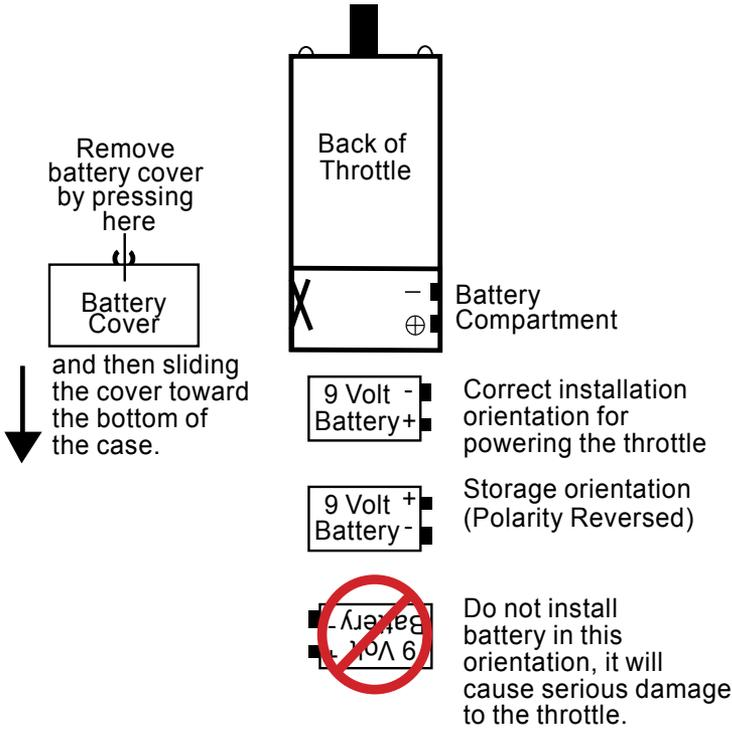
For normal walk around (tethered) operation, the DT402 series throttles do not need a battery. However, when you are unplugged from LocoNet, your throttle display will go off. We recommend using a battery for DT402 operation even though it is not required. To use your DT402/R/D as an infrared or radio throttle, you must install a 9-volt battery. When you install the battery, the throttle will report the battery voltage then show the last display screen used by the throttle.
