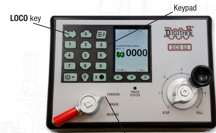
Direction/Brake lever in “FORWARD” position
