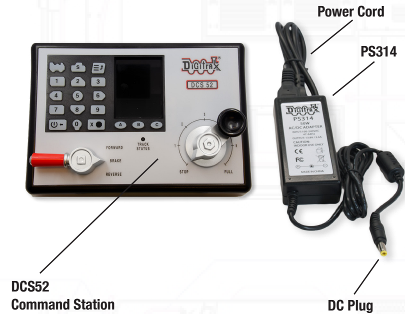
Direction/Brake lever in “BRAKE” position
