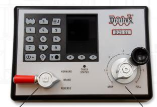
**Direction/Brake** lever in "BRAKE" position
