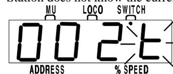
This display example shows Switch #2 is in an unknown position.
