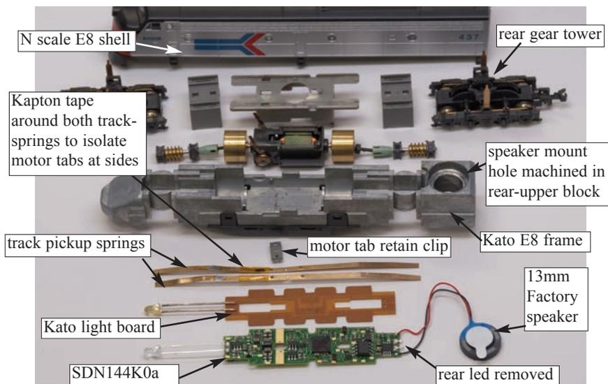
1. Carefully remove the Kato E8 shell. Remove the analog light board, trucks, gear towers drive shafts, motor and all parts and carefully save these parts in the correct order for re-installation. This should leave a bare frame ready to be modified to accommodate the speaker. Isolate the track pickup springs from the motor tabs using supplied Kapton tape.
