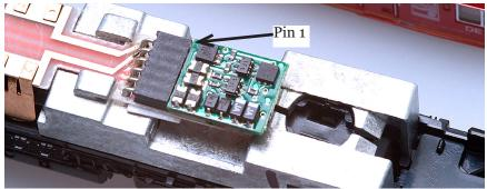
Figure 2: Kato N-EMD class 66 with DZ126IN installed
