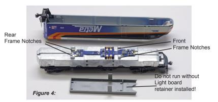
4. Install the DN163K4B decoder by tilting it slightly down at back as you insert the decoder into the rear frame notches. <u>Carefully</u> maneuver the decoder motor tabs down over the motor contacts and then level and slide the decoder board backwards so the board's corners are under the front
