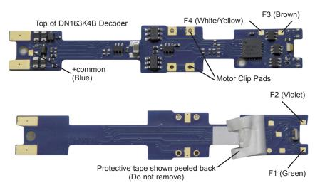
Figure 6: Connecting More Functions to Your DN163K4B Decoder
