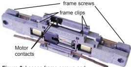
Figure 2: Loosen frame screws and remove light board
