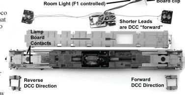
in the forward end and red in the rear end when the loco is running forward. The lights will automatically change when the loco is reversed.
