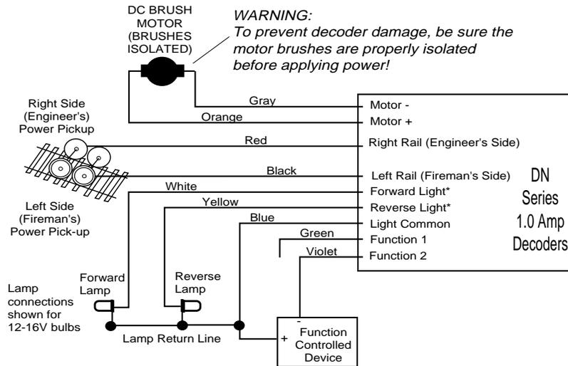
\* Forward and reverse lights can be run as independent functions on F0 & F4. See CV61 in chart on previous page and see Digitrax Decoder Manual for Complete Instructions.
