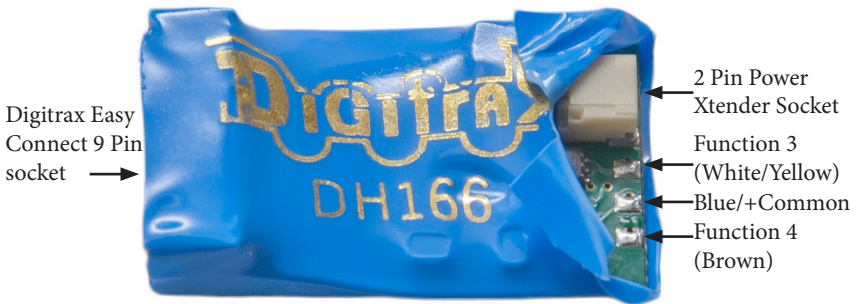
Figure 5. DH166D Decoder Function Outputs
