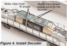
Spread Motor clip pins if necessary. Motor Clip pins must fit snugly into decoder PCB!
