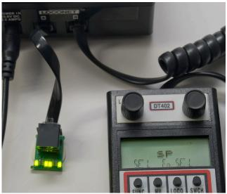
9. If any of the LEDs fail to glow or are dim, cut the ends off the cable and crimp new connectors on the cable. Re-test the cable. If it still fails the test, there may be a problem with the cable itself and you should consider discarding it. 10. DO NOT leave the LT1 connected to a running layout, because it adds an extra unnecessary load to LocoNet. It is meant to be used as a simple temporary diagnostic tool only.
