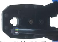
Step 4: Position RJ12 Plug and prepared cable.
