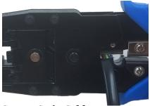
**Step 3: Strip Cable**Squeeze the handle and pull the tool keeping the cable perpendicular to strip off outer insulation without damaging the insulation on the inner wires.
