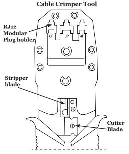
the pin 1 position. Make sure that the inner wires are flush with the tip of the connector and directly under the gold contacts, squeeze the handles FIRMLY to set the contacts and secure the cable, thus completing the operation.
