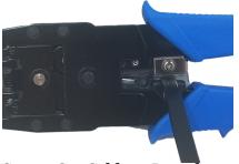
**Step 1: Cut Cable to Length**Cut the LocoNet cable to the desired length. Make sure that the ends are cut squarely, not diagonally.
