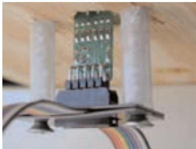
Here the Signal Mast Base is plugged into a Signal Driver Cable's Socket which is mounted under the layout using Signal Spacers and Metal Signal Installation Straps. Notice that here, we used two signal installation straps to hold the signal driver cable and socket in place.
