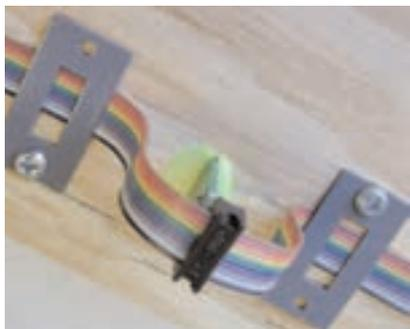
Here two Metal Signal Installation Straps are used to hold the Signal Driver Cable's Socket in place. The Signal Mast Base is inserted through a hole in the layout and the hole is filled with clay to hold the signal mast upright. In this case, the socket is floating to allow some "wobble room" in case the signal is disturbed during operation.
