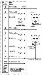
Wiring for A<sub>1</sub> (main) and A<sub>2</sub> (diverging or dwarf)
