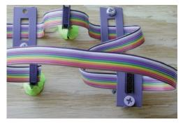
Here Metal Signal Straps are used to twist the Signal Driver Cable under the layout to position the sockets in the proper orientation for signal installation. The last socket on the Signal Driver Cable is held in place with clay alone.
