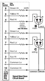
Wiring For B (main) and C (siding)
