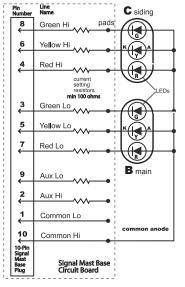
Wiring for A<sub>1</sub> (main) and A<sub>2</sub> (diverging-dwarf)
