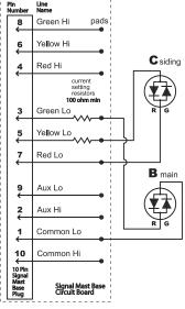
Wiring for A<sub>1</sub> (main) and A<sub>2</sub> (diverging or dwarf)
