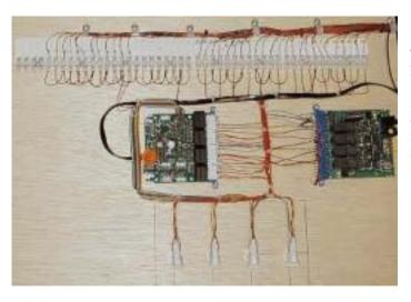
This photo shows the required spacing for the installation of one PM42, one BDL168 and one RX4. Each RX1 on your RX4 should be installed at least 2 inches from any other RX1. All RX1s should be installed in the same orientation relative to each other. Wires should be routed as shown to avoid interference that might cause problems with operation of detection. More information about spacing is presented later.
