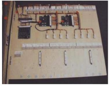
This photo shows an example wiring panel with one PM42, two BDL168s and two RX4s installed and labeled terminal strips on the upper half of the board.
