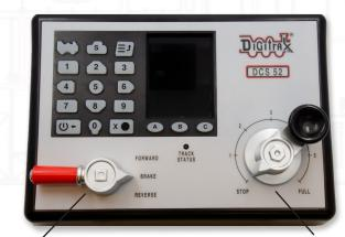
**Direction/Brake** lever in "BRAKE" position
