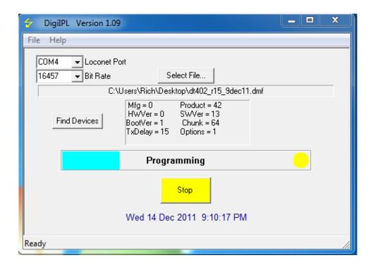
While the device is being updated, various LEDs will blink. If updating a Throttle, the white Flashlight LED will blink and the Throttle Display will display 'IPL Run'
