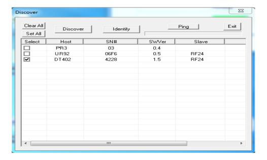
In this example, the PR3 has version 4, UR92 has version 5 and the DT402 has version 1.5 loaded.
