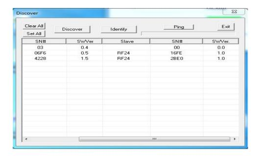
If the FAR Right **SWVer.** Column reads **1.0**, the RF24 Duplex Radio Module has updated correctly.
