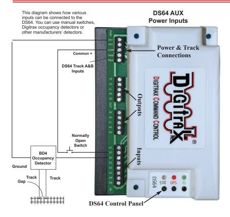
Figure 4: Connecting Input Devices to Your DS64
