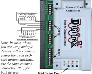
This diagram shows how sole-noid and bi-polar machines can be connected on your layout. You can use any combination of machine types shown here.
