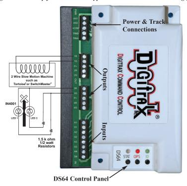
Note: Multiple turnout machines can be operated on a single DS64 output. For example, you can run 2 Tortoise or Switchmaster machines on a single DS64 output.
