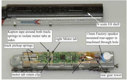
Figure 2: SDN144K0a Decoder installation in Kato E8 - reassembled.
