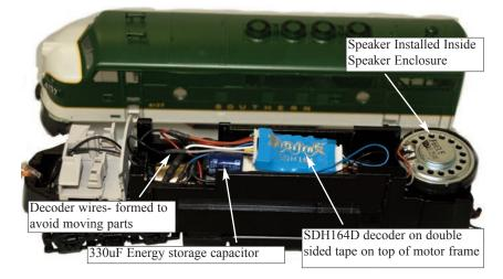
Figure 2: SDH164D: installation example in an Athearn Diesel
