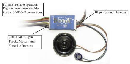
SDH164D showing 10 pin sound harness with 32ohm 28mm Speaker, 330uF Capacitor
