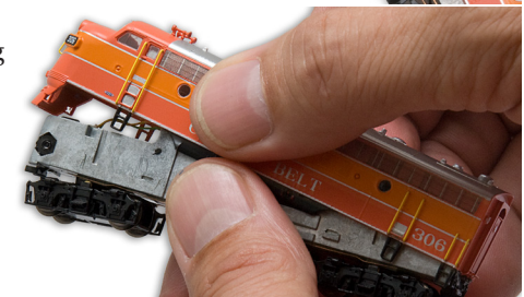
Figure 2: Grasp toothpicks and gently remove shell from frame.
