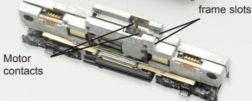
**Figure 2:** Loosen frame screws and remove light board
