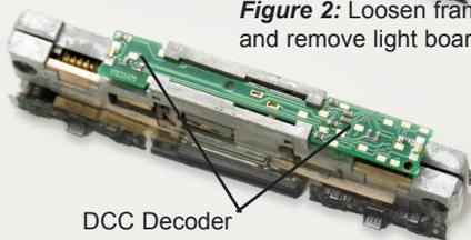
**Figure 3:** Place decoder in frame.
