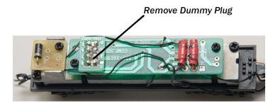
Plug DN146IP into socket as shown.
