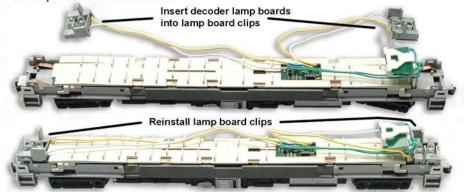
10. Test decoder for correct operation. Once test is completed, replace loco shell.
