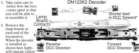
in the forward end and red in the rear end when the loco is running forward. The lights will automatically change when the loco is reversed.
