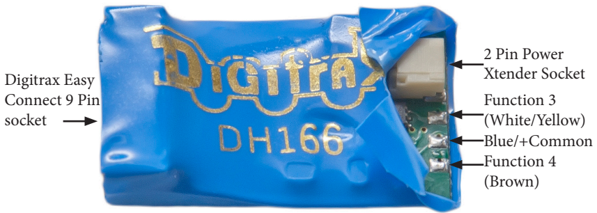
Figure 5. DH166PS Decoder Function Outputs
