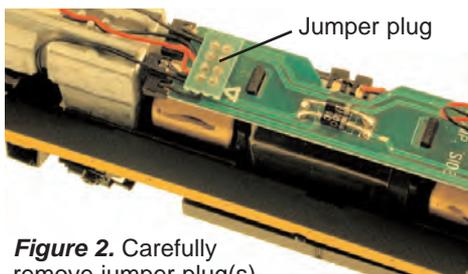
**Figure 2.** Carefully remove jumper plug(s)
