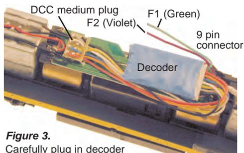
**Figure 3.** Carefully plug in decoder
