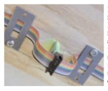
Here two Metal Signal Installation Straps are used to hold the Signal Driver Cable's Socket in place. The Signal Mast Base is inserted through a hole in the layout and the hole is filled with clay to hold the signal mast upright. In this case, the socket is floating to allow some "wiggle room" in case the signal is disturbed during operation.
