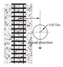
1. Locate the placement of your signal mast on the layout and drill a 5/8" hole through the sub-roadbed next to the track road bed. This will allow the signal mast base to pass through the layout table. The distance (*x* in the following diagram) from the center of the track to the signal will be different for each prototype railroad and each model scale.
