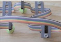
Here Metal Signal Installation Straps are used to twist the Signal Driver Cable under the layout to position the sockets in the proper orientation for signal installation. The last socket on the Signal Driver Cable is held in place with clay alone.
