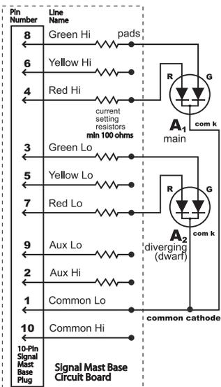
Wiring for A<sub>1</sub> (main) and A<sub>2</sub> (diverging or dwarf)
