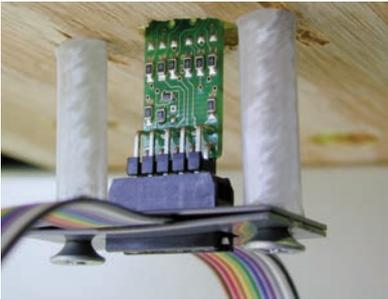
Here the Signal Mast Base is plugged into a Signal Driver Cable's Socket which is mounted under the layout using Signal Spacers and Metal Signal Straps. These components are available in the Signal Mounting Hardware Kit which consists of 6 Straps and 6 Spacers..
