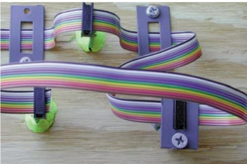
Here Metal Signal Straps are used to twist the Signal Driver Cable under the layout to position the sockets in the proper orientation for signal installation. The last socket on the Signal Driver Cable is held in place with clay alone.
