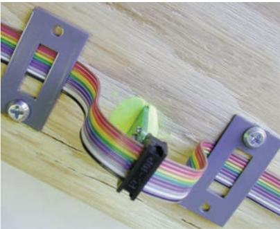
Here two Metal Signal Straps are used to hold the Signal Driver Cable's Socket in place. The Signal Mast Base is inserted through a hole in the layout and the hole is filled with clay to hold the signal mast upright.
