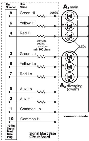
Wiring for A<sub>1</sub> (main) and A<sub>2</sub> (diverging-dwarf)
