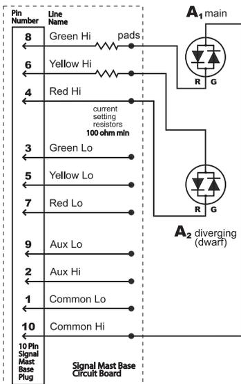
Wiring for A<sub>1</sub> (main) and A<sub>2</sub> (diverging or dwarf)
