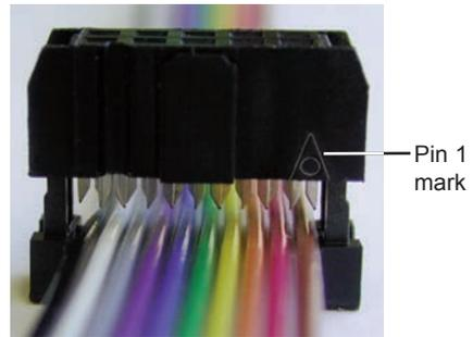
4. Place the top part of the connector, metal pins toward the cable, over latches on the bottom part of the connector. The Pin 1 indicator arrow on the side of the connector should be over the brown wire.
