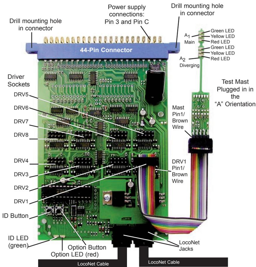
LocoNet Jacks-Use LocoNet cables to connect to Command Station/Throttle or PC with control software
