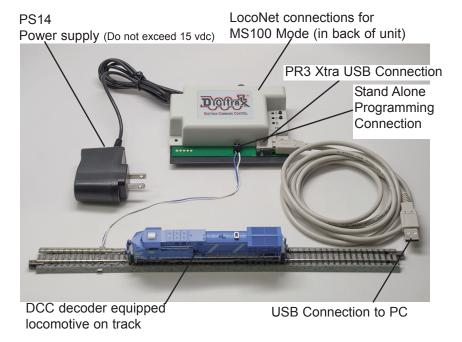
The connection diagram on the following page will help you install the hardware correctly. Assemble the PR3 Xtra hardware as shown and connect to the Digitrax PS14. Input voltage to the PR3 Xtra should not exceed 15vdc otherwise damage to your sound decoder may occur. Note for MS100 mode, the PR3 Xtra must be connected to the Command Station with LocoNet. For Stand Alone programming, no LocoNet connection is required.
