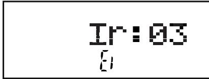
This display shows a DT400 that has found an Infrared receiver on LocoNet with a current LocoNet ID of 03. The DT400 is ready to Edit the LocoNet ID. Other characters may be displayed on the screen at this time depending on the current throttle state.
