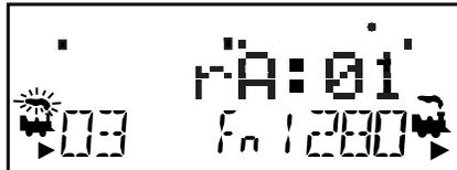
4. The DT400R/DT402R will use the **LocoNet ID** of the LocoNet it was plugged in to and will begin to operate as an IR throttle when you unplug it from LocoNet. When you unplug from LocoNet, the tetherless indicator will come on and the tetherless message will display for a few seconds indicating whether the throttle is running as Ir (infrared) or rA (radio). It will also display the LocoNet ID that the throttle is logged on to.
