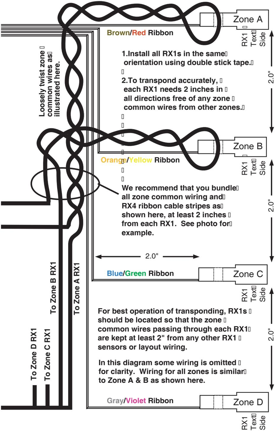
1. Install all RX1s in the same orientation using double stick tape.
