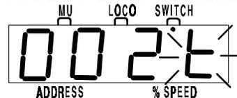
This display example shows Switch #2 is in an unknown position.
