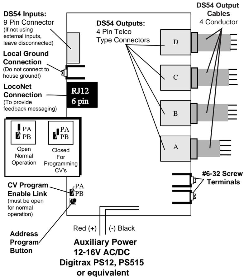
**DS54 Outputs:** The four outputs for the DS54 are four telephone type connectors labeled A, B, C & D. These are 4 pin connectors and are used to link the DS54 to the turnout machines or other layout devices controlled by the DS54.
