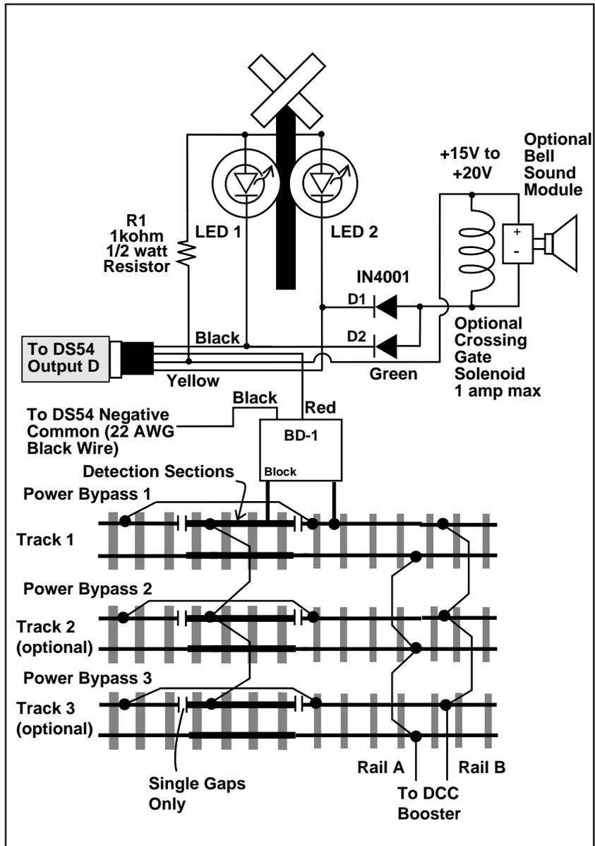
Figure 14: Automatic crossing gate with multiple detection sections
