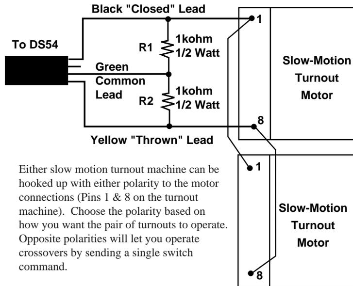
Either slow motion turnout machine can be hooked up with either polarity to the motor connections (Pins 1 & 8 on the turnout machine). Choose the polarity based on how you want the pair of turnouts to operate. Opposite polarities will let you operate crossovers by sending a single switch command.
