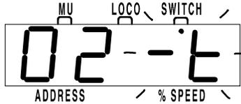
3. Use either throttle knob or the up and down arrow keys to scan to the switch address that you want to change. DT100s use the three left digits to display the switch address and DT200 throttles use the two left digits to display the switch address.
