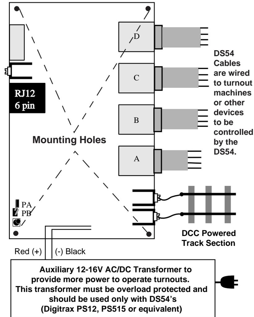
*Figure 6: Hooking up solenoid turnout machines.
