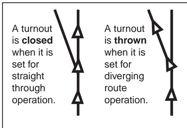
*Figure 1: Turnout Position, Closed & Thrown*
