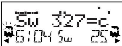
This display example shows Switch Address Number 327 is in the closed position.
