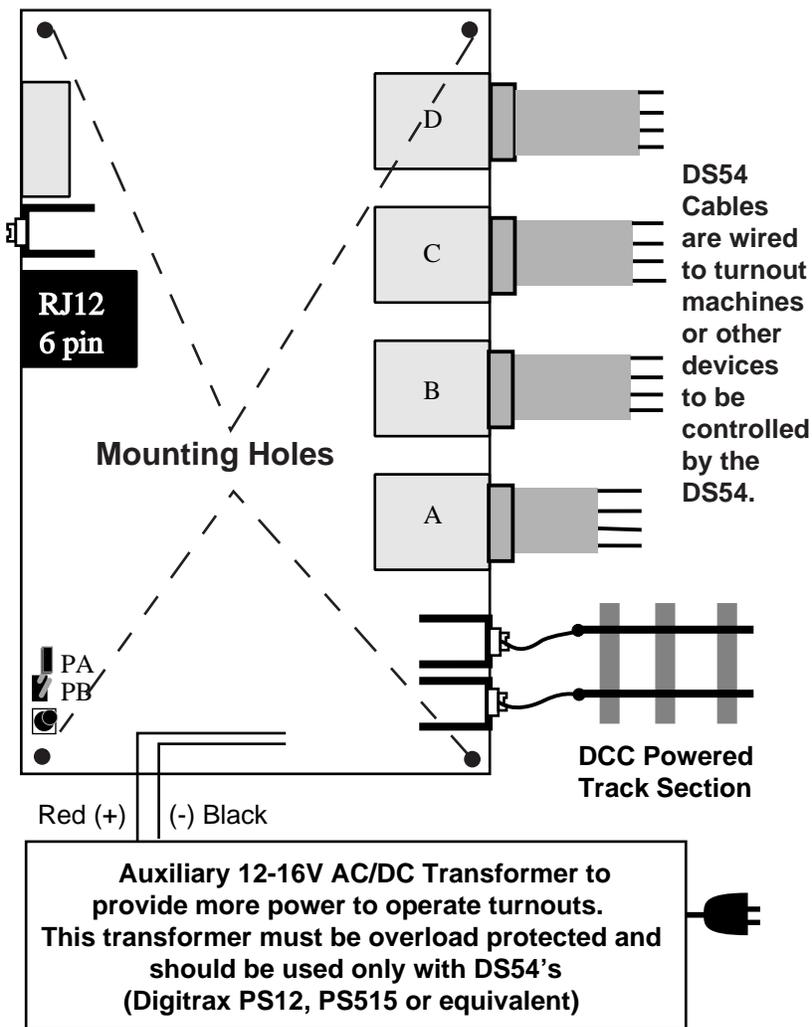
*Figure 6: Hooking up solenoid turnout machines.
