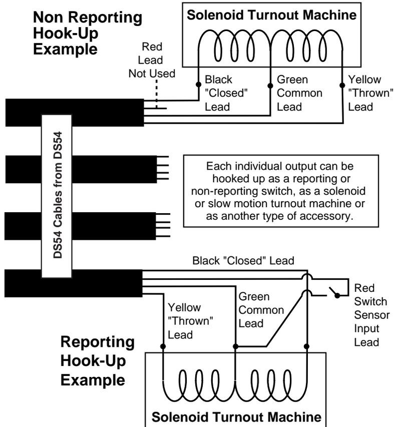
If you are not using reporting, simply leave the red switch sensor input lead unconnected.
