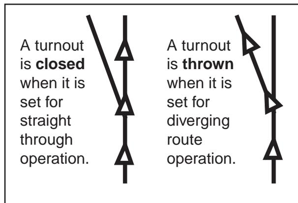
*Figure 1: Turnout Position, Closed & Thrown*
