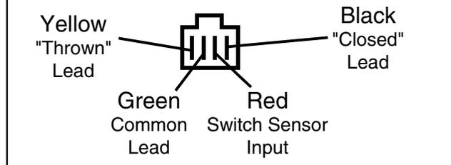
**DS54 Inputs:** The 9 pin Digitrax connector is used on the DS54 for inputs from devices on the layout. These inputs can be from things like momentary contact switches for determining turnout position, from BD1 occupancy detectors or other devices. Each function cell has a pair of input wires available.
