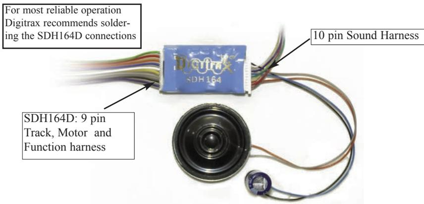
SDH164D showing 10 pin sound harness with 32ohm 28mm Speaker, 330uF Capacitor
